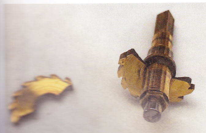
Figure 4. The repair on the broken ratchet wheel.
